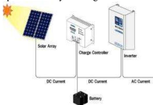
Gambar 2. Sistem Energi Surya Fotovoltaik
